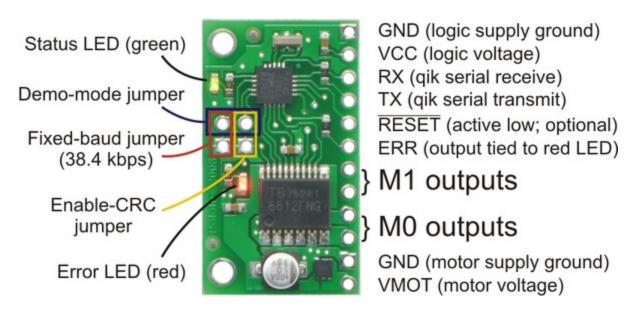
The qik connections are shown above, and most of the pins are labeled on the back side of the motor controller. All square pads are ground.
