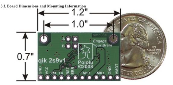
The qik 2s9v1 measures  $0.7" \times 1.2" \times 0.28"$  ( $17.8 \times 30.5 \times 7.1$  mm) and weighs 0.07 oz (2.0 g) without the header pins installed. It has two mounting holes, one in each top corner. The holes have a diameter of 0.086" and are designed for #2 or M2 screws.
