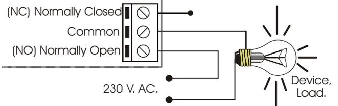
**INFORMATION ABOUT THE OUTPUT.** During the operating mode and according to its load, it could happen a fluctuation or an incorrect working of the output. In such case, you have to install an anti-spark circuit between both contacts of the used relay, as it is indicated on the schedule.
