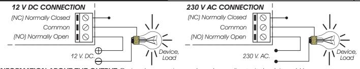
**INFORMATION ABOUT THE OUTPUT.** During the operating mode and according to its load, it could happen a
