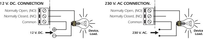
**INFORMATION ABOUT THE OUTPUT.** During the operating mode and according to its load, it could happen a fluctuation or an incorrect working of the output. In such case, you have to install an anti-spark circuit between both contacts of the used relay.
