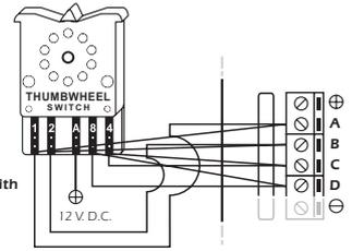
Pic. 1. How to connect the display with a BCD Preselector BCD.
