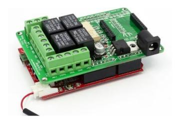
Step1. Plug Relay Shield onto Arduino Duemilanove (or compatible) board;
