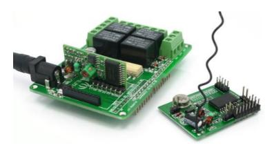
Step1. Plug the Receiver onto the Relay Shield.
